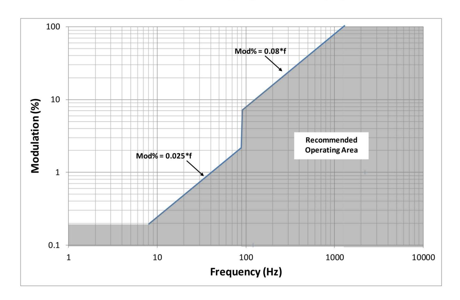
NOTE—Operating in the shaded area minimizes visual discomfort or annoyance and also gives low risk for headaches and photosensitive epileptic seizures. Below 90 Hz, Modulation (%) is less than 0.025×frequency. At or above 90 Hz, Modulation (%) is below  $0.08 \times$  frequency. Modulation (%) =  $100 \times (Lmax - Lmin)/(Lmax + Lmin)$  where  $L_{max}$ , and  $L_{min}$ correspond to the maximum and minimum luminance, respectively. The figure was derived from the low-risk regions in Figure 18.
